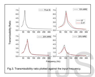
Under the influence of the magnetic field, the embedded iron particles gets aligned in the direction of flux lines which results in enhancement in the properties. In the current experiment, the loss factor of pure Silicone sample was found to be 0.132 and the 25% MRE sample 0.235 showing an improvement of about 75%.
